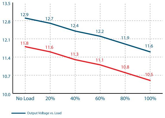
Output Voltage With a Typical Dimmer
