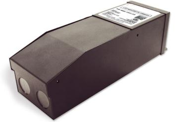
KLUS - MD-200-12 is the most compact LED driver on the market with a magnetic transformer core. It is equipped with two push-to-reset circuit breakers on the input and output, which protect both the load and driver. The driver is encased in a coated metal box that includes 2 knock-outs on the bottom to enable easy installation that complies with electrical code requirements.
